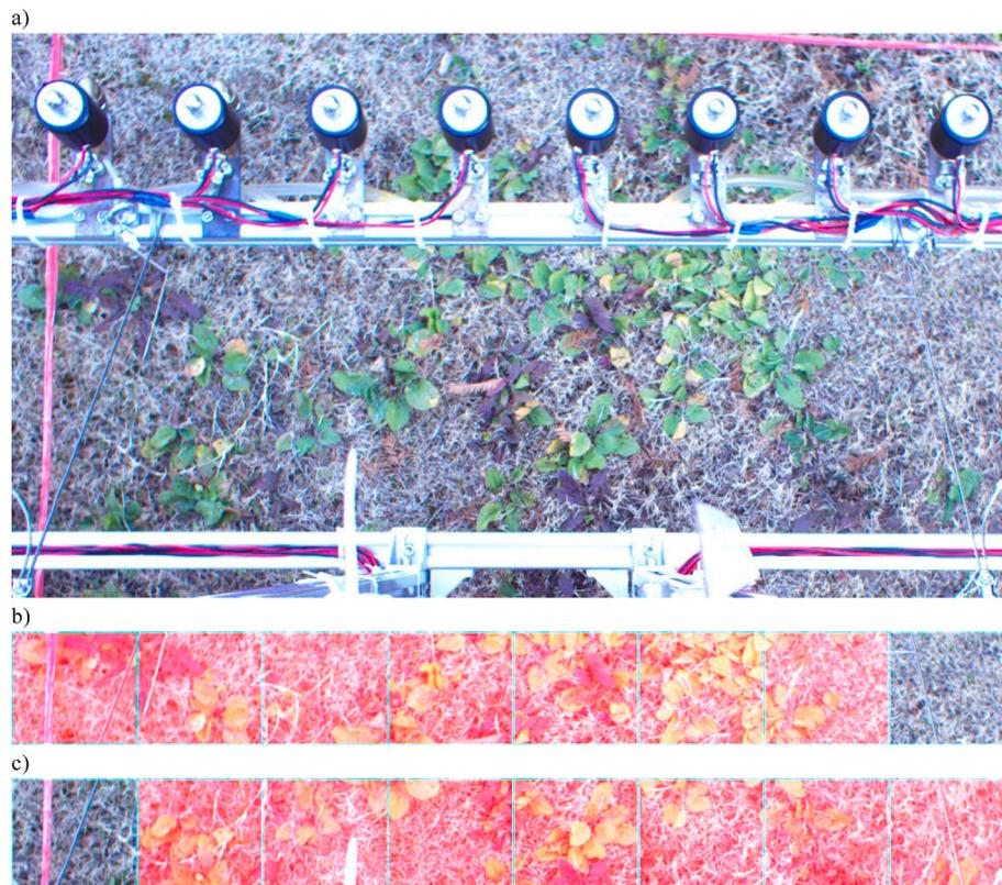
**Fig. 4.** Weed detection and localization results. The original image ( $1920 \times 1080$  pixels) was captured by the machine vision system (a), ROI 1 and ROI 2, and the neural network successfully predicted the grid cells ( $240 \times 216$  pixels) containing weeds while growing in dormant bermudagrass turf (red) (b, c). Abbreviation: ROIs = regions of interest. (For interpretation of the references to color in this figure legend the reader is referred to the web version of this article).
