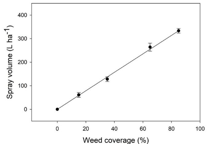
Fig. 5. Herbicide spray volume depends on the weed coverage when using the developed smart sprayer prototype for precision herbicide application. Data were analyzed with linear regression equation  $y = -1.394 + (3.965 \times x)$ , where  $y$  represents spray volume (L ha<sup>-1</sup>) and  $x$  represents visual weed coverage (%).
