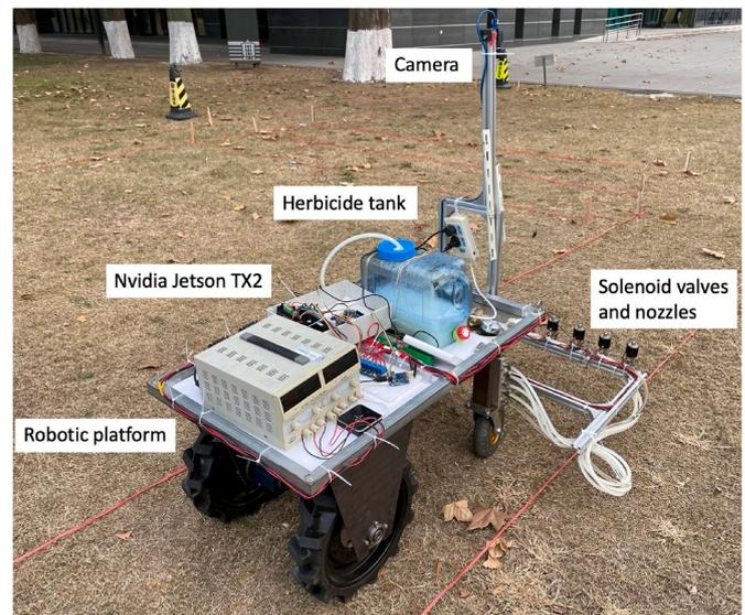
Fig. 1. Main components of the smart sprayer prototype.
