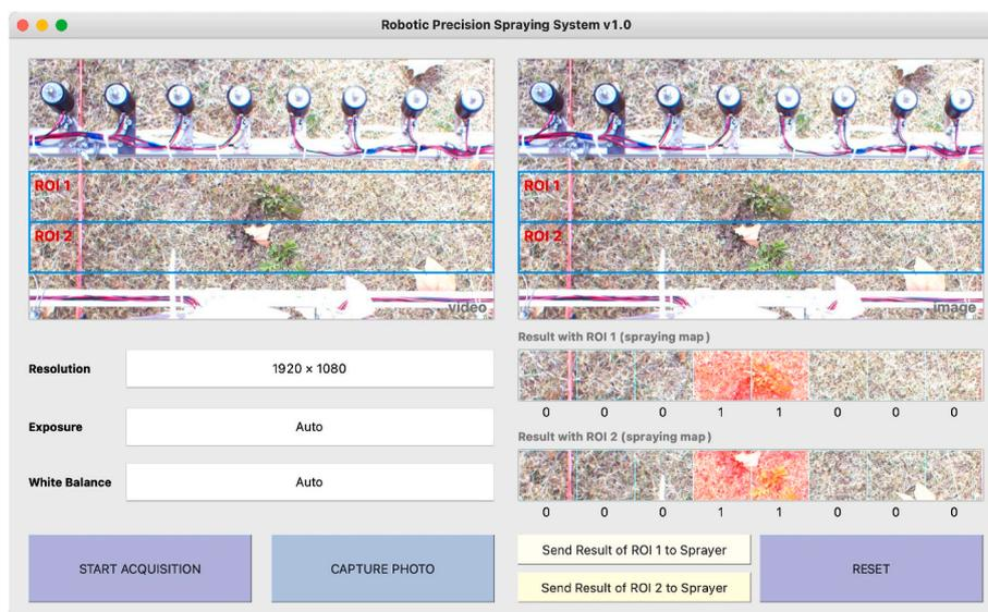
Fig. 3. Graphical user interface displays video streaming and processes the captured images. The grid cells of ROIs were highlighted as red color when the interference indicated they contained weeds. Abbreviation: ROIs = regions of interest.
